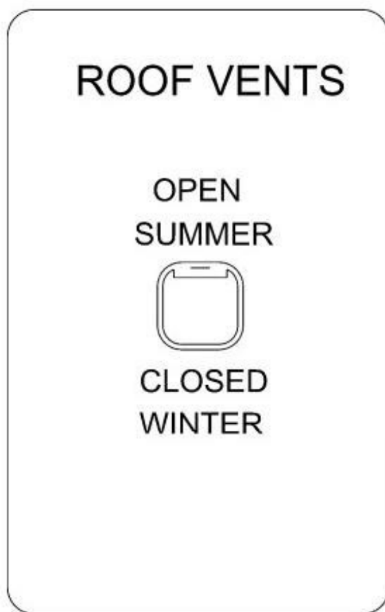
Figure 07: Typical Switch Layout for Damper Operation for Roof Ventilators
